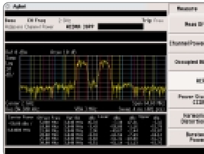
Six offsets in the ACPR measurement allow rapid assessment of components that handle multicarrier signals.
